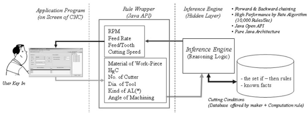
Fig. 5. Cutting condition recommendation system using rule-based knowledge Base.
