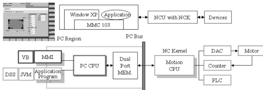
Fig. 3. Structure of open CNC controller.
