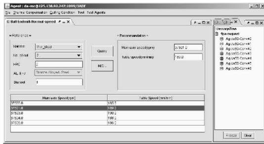
Fig. 6. Recommendation of cutting conditions for common processes.
