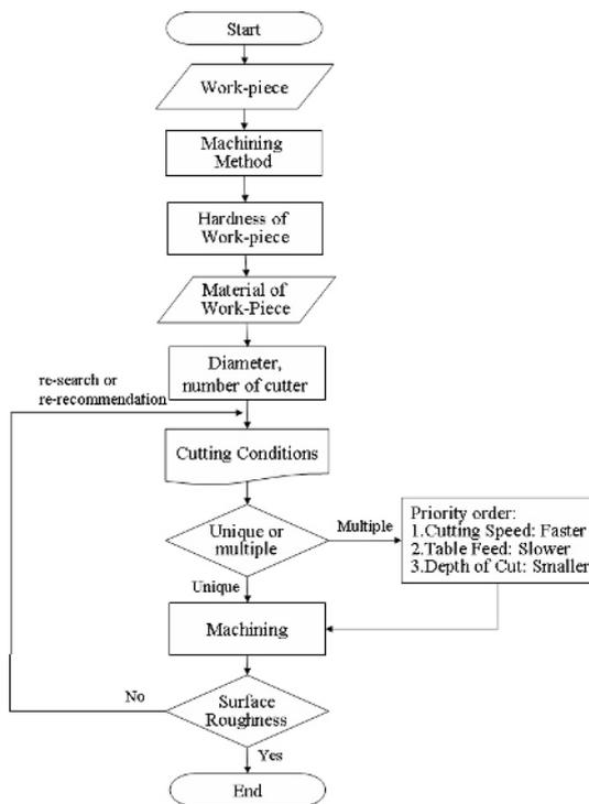
Fig. 2. Flow diagram of optimal cutting conditions for ball-end milling.
